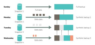
Figure 2. Incremental and synthetic full backups
